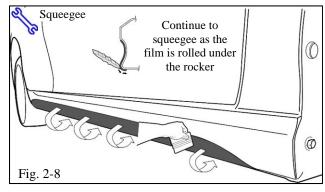
(f) Remove the bottom section of the liner and squeegee the part onto the rocker starting from the top edge. Continue to squeegee the applique along the length of the vehicle along the recessed area (Fig. 2-6).
