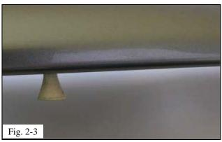
NOTE: To assist in the alignment of the applique, a golf tee may be inserted into the drain hole of the rocker. Align the drain hole cutout on the applique against the golf tee (Fig. 2-3 and Fig. 2-4). Remove the golf tee upon completion of step.
